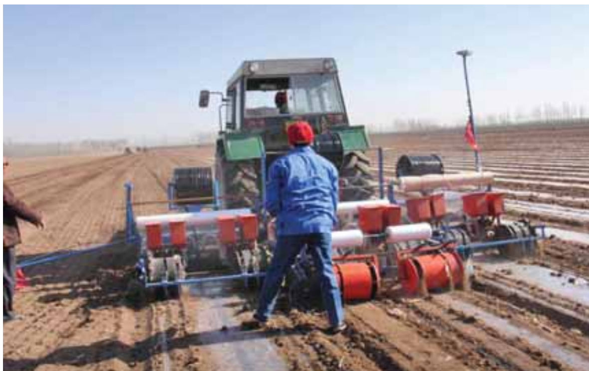
Figure 8: Multiple function equipment for planting and applying plastic film mulch
